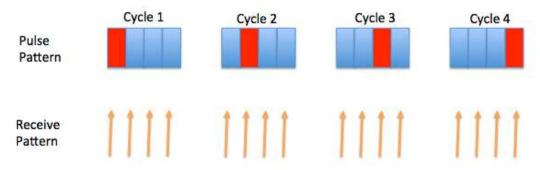
Figure 1. Pulse/receive pattern for a FMC acquisition using a linear array with four elements.
